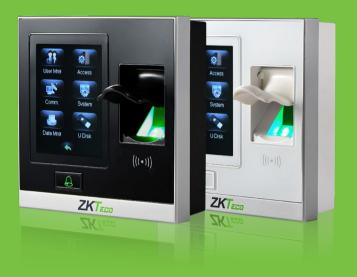
SF400 is an IP based fingerprint terminal with both Network and Standalone operation modes. It is connectible with ZKBio CVAccess software for access control and time attendance management.
